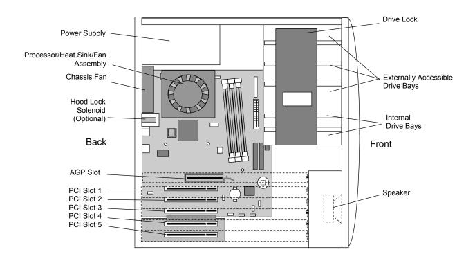
Figure 2–6. Configurable Minitower Chassis Layout, Left Side View (Minitower configuration)
